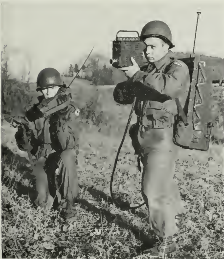
During demonstration at Fort Monmouth, N. J., soldiers equipped with RCA-built portable TV transmitter and transceiver radio send data to headquarters.
